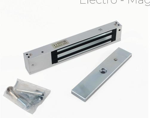
An electromagnetic lock, 'magnetic lock', or 'maglock' is a locking device that consists of an electromagnet and an armature plate. Direct pull electromagnetic locks are inherently fail-safe.
