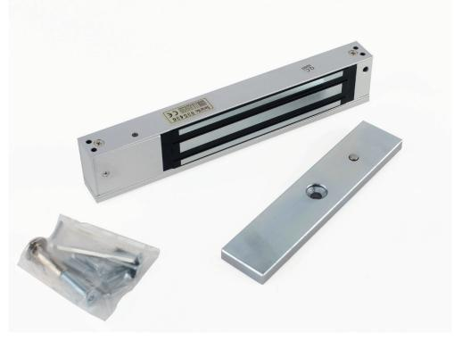
An electromagnetic lock, 'magnetic lock', or 'maglock' is a locking device that consists of an electromagnet and an armature plate. Direct pull electromagnetic locks are inherently fail-safe.
